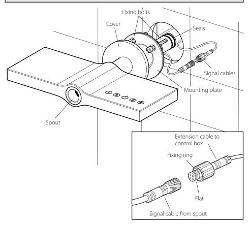
Flush through the pipe work to ensure removal of debris, turn off the water supply. Unscrew the cover and slide forwards to access the mounting plate and bolts.
