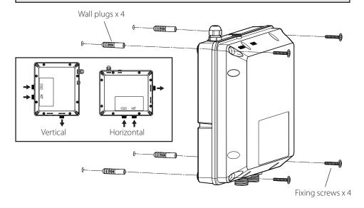
The Control box can be installed either vertically or horizontally (see above).
