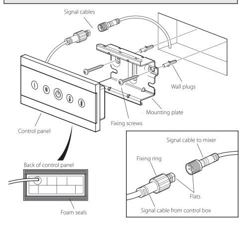
In the required position prepare a recess in the wall 112mm x 42mm and by 23mm deep.
